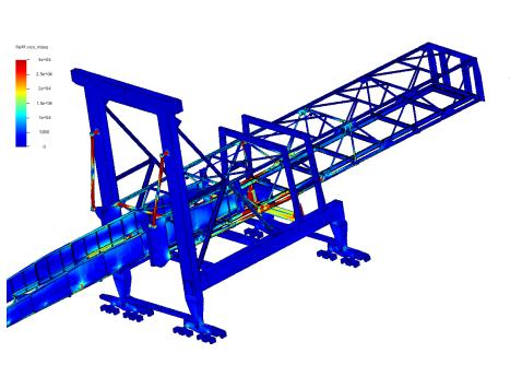
Next-generation software for high-speed and very accurate computer-based simulations of very large and complex mechanical structures
